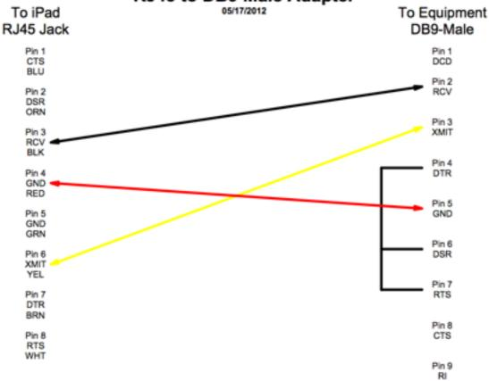
Note: This adapter is designed to be used with the Redpark iPad Console Cable and Get Console App
