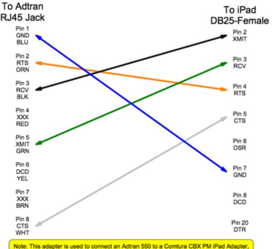
Note: This adapter is used to connect an Adtran 550 to a Comtura CBX PM iPad Adapter, which in turn connects to a Redmark iPad Console Cable
