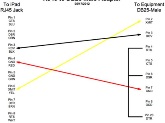
Note: This adapter is designed to be used with the Redpark iPad Console Cable and Get Console App
